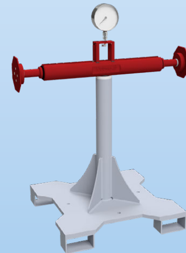
Test equipment available: hydraulic test jack
